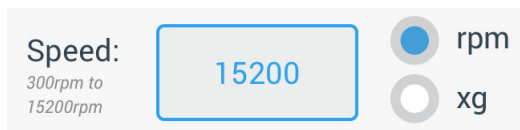
Figure 3-15: Setpoints Screen Detail for Centrifuge Speed, and Range
