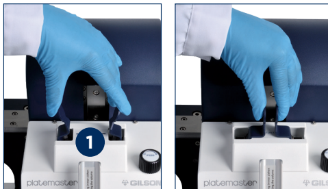
Figure 11 Tip ejection system
