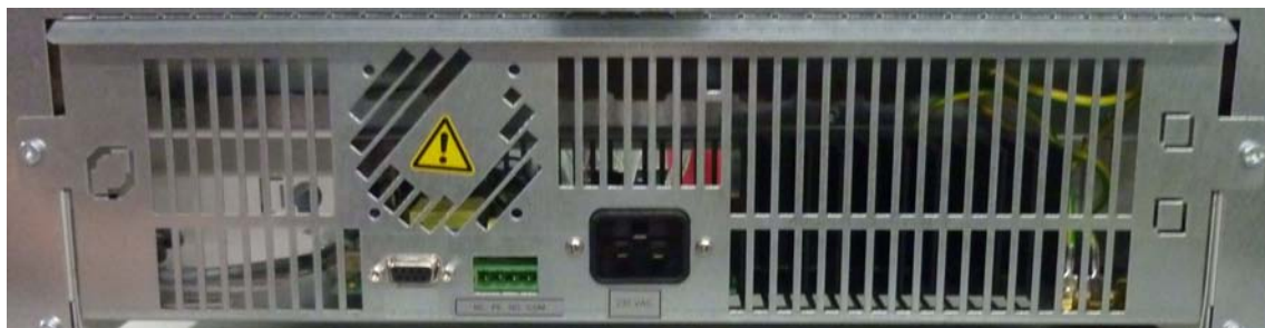
Figure 5-10 AC Power Supply Socket
