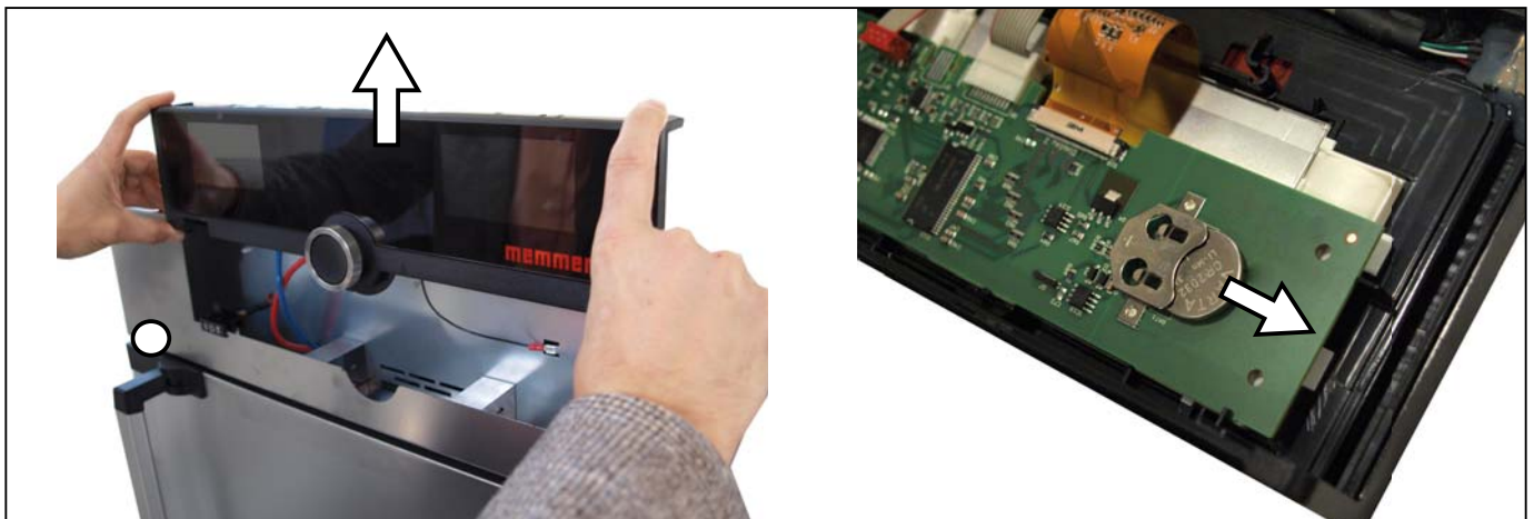
Fig. 32 Removing the lithium battery
