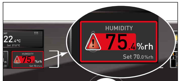
Fig. 21 Humidity monitoring triggered
