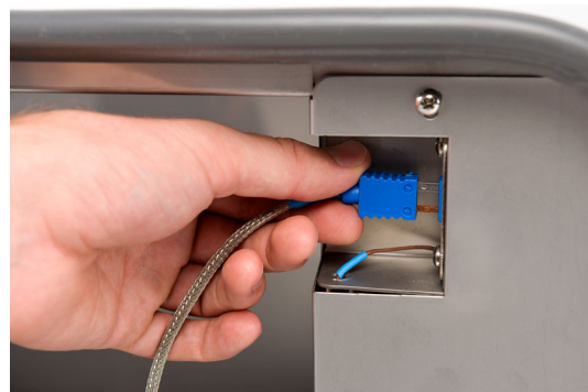
Figure 4. Sample Thermocouple Connection
