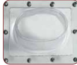
Microscopes become more valuable tools for intrachamber work with the use of this optically clear flexible vinyl sock. The sock is sealed to the chamber wall and is installed directly over the microscope's eyepieces, enabling easy use of the oculars. This accessory is recommended particularly for chambers with more than
