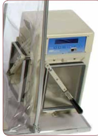
Coy vacuum airlocks (manual or automatic) remove O<sub>2</sub> from ambient conditions to achieve acceptable levels of O<sub>2</sub> prior to transfer to/from the chamber. The airlock reaches the low O<sub>2</sub> level through a multiple vacuum/purge procedure. The standard factory procedure is to pull a vacuum to 20" of mercury, then purge back to 1" of Hg using an inert background
