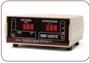
This patented analyzer constantly monitors both oxygen and hydrogen levels within a chamber at a fraction of the cost of two separate analyzers. The unit monitors both oxygen and hydrogen directly from the chamber atmosphere. The analyzer's constant
