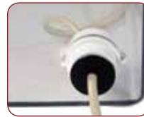
One feed-thru adaptor (1½ "/38 mm) is supplied as standard to meet customer needs for electrical wiring, tubing or any type of cord that needs to be sealed through the chamber wall. Customers may order additional feed-thru adaptors as factory-installed options.
