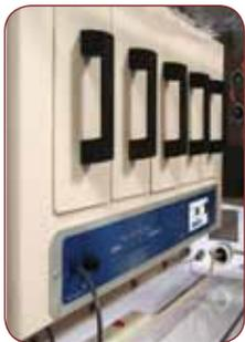
The incubators for rigid chambers are sturdy wall-mounted units with five pull-out drawers for holding specimens for incubation. Each drawer features a system of slots, cavities and brackets for positioning petri dishes and well plates and securing them in place. The Model 2002 is equipped with solid-state electronics that allow precise monitoring and control of heat output. A bright LED digital display provides a readout of the incubator's
