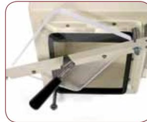
This update to the airlock door has a spring-loaded corner pivot which allows the door to swing up while parallel to the airlock, saving valuable space. Older Coy airlocks may be retrofitted in the field with the new style door and updated digital electronics.
