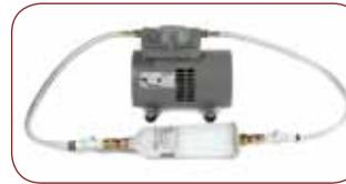
This system filters the chamber atmosphere and controls contamination by particles 0.3 micron and larger. The external pump-activated system has the filter mounted outside of the chamber.
