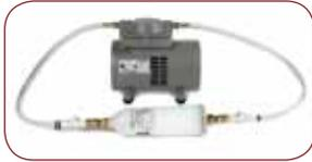
This system filters the chamber atmosphere and controls contamination by particles 0.3 micron and larger. The external pump-activated system has the filter mounted outside of the chamber. The system draws the internal atmosphere out of the chamber, through the external filter and back into the chamber. Equipped with
