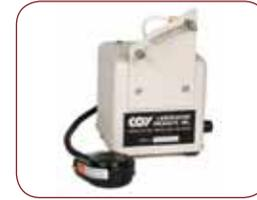
Flaming a bacteriological loop and the edge of a culture tube inside a chamber is easy with Coy's incandescent flaming device. The flaming unit is plugged
