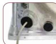
Two feed-thru adaptors (2"/51 mm and 1½"/38 mm) are supplied as standard to meet customer needs for electrical wiring, tubing or any type of cord that needs to be sealed through the chamber wall. Customers may order additional feed-thru adaptors as factory-installed options.
