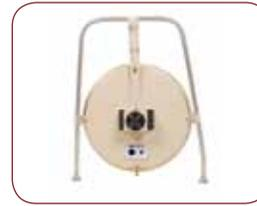
This easy-to-maintain unit is used in highmoisture-content vinyl anaerobic chambers and provides a way to remove moisture without using a desiccant. The dehumidifier operates as a simple cold wall to condense moisture from the air; a drain removes excess moisture from the chamber.
