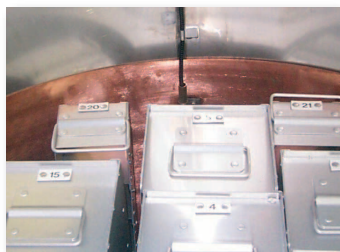
Super Chill accessory lowers temperature and provides near isothermal storage at -190°C
