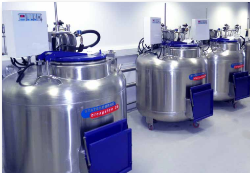
Three Biosystem 40 units provide fully automated storage for over 44,000 specimens each in vapour phase with dependable temperature stability at -185°C (Plus/minus 4°C)
