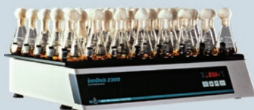
Innova 2300 Maximum flask size: 6 L Orbit: 2.5 cm (1 in) or 5.1 cm (2 in)
