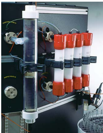
Fig 10. Four HiPrep 26/10 Desalting columns connected in series.
